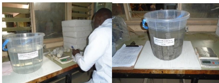
Figure 2.6: Water Absorption (24Hour Soak) Porosity Measurement
