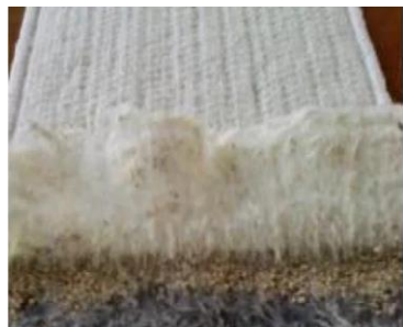
Figure 5: Geosynthetics Clay Liner -Civilblog.org
