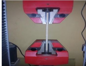
Figure 1: Tension Test arrangement
