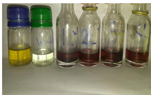
Plate 1b. Synthesized Ag-AuNPs containing 4ml of Silver and Gold and 0.5ml, 1ml, 1.5ml and 2ml extract of Dioscorea respectively Extract Ag- Au 2ml 1.5ml 1 ml 0.5ml
