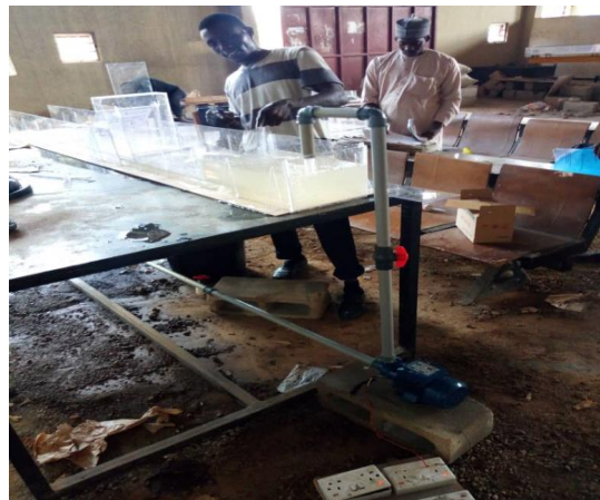
Fig. 5: observation of water level above the vertex of the v-notch weir.
