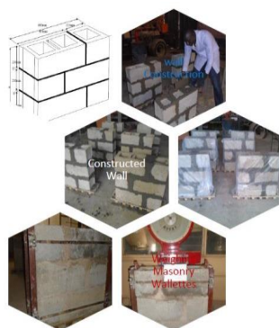
Figure 5: Masonry Hollow Concrete Block Wallette's
