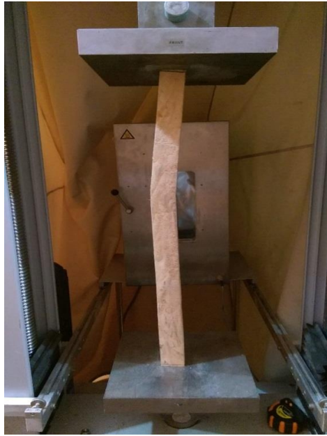
Figure 3: Failure mode of 200mm (Buckling)
