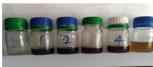
Plate 1c. Synthesized Ag-AuNPs containing 4ml of Silver and Gold and 0.5ml, 1ml, 1.5ml and 2ml extract of Solenum Tuberosum respectively Extract Ag-Au 0.5ml 1ml 1.5ml 2ml
