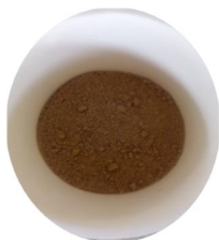
Plate 5: Formulated Batch composed of 95.899g of SCBA, 19.220g of CaCO 3 and 25.556g of Na 2 CO 3
