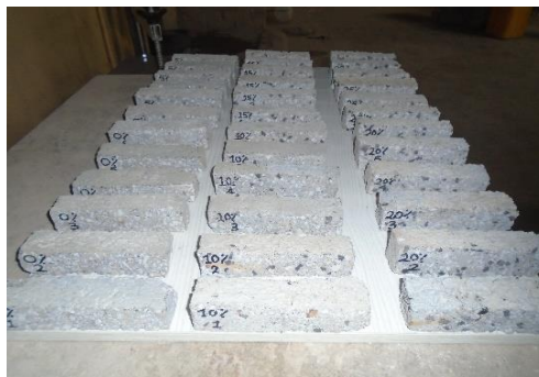
Figure 2.3: Masonry Concrete Samples for Sorptivity and Porosity Test
