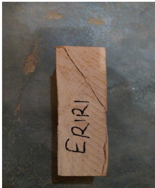
Figure 2: Failure mode of 200mm (Splitting)
