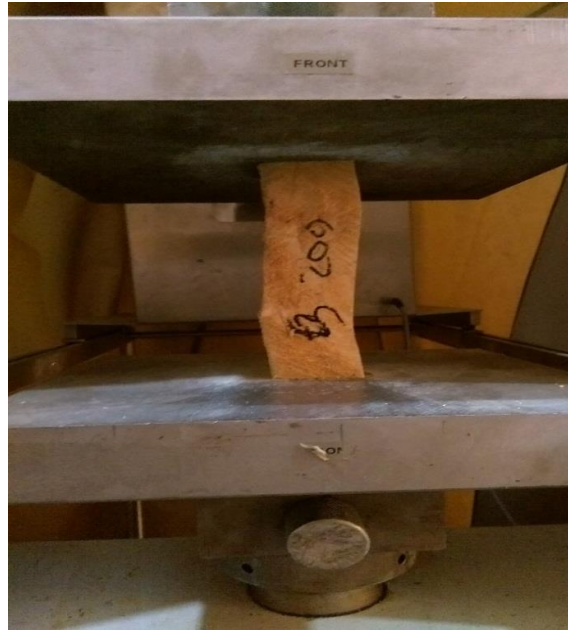
Figure 1: Failure mode of 200mm (Shear)
